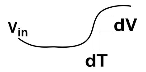
Fast signal converts a sample timing error (dT) to an apparent voltage error (dV).
